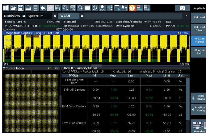
Analysis of a 320 MHz wide and 4096QAM modulated WLAN 802.11be signal using the R&S®FSW-K91BE option
