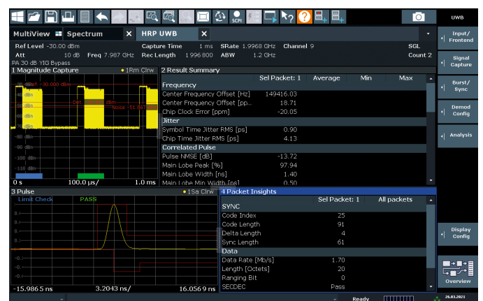
HRP UWB signal analysis with the R&S®FSW-K149 high rate pulse repetition frequency ultrawideband measurement application
